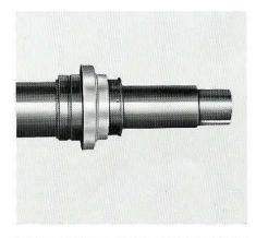
Packing sleeve—The packing sleeve is centrifugally cast Type 316S/S, coated with ceramic and given a precision polish. Alternate sleeve materials are available.
