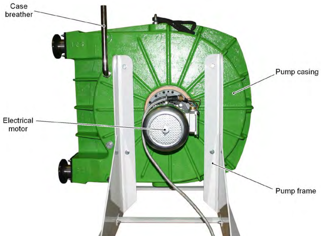
Fig 2 VF125 Pump unit (rear view)
